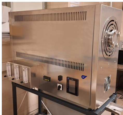
High-temperature atmospheric tube furnace Czylok, Poland
