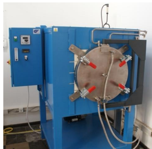
Programmable, atmosphere furnace Czylok FCF-V70C/R
