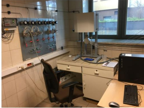
Electrochemical reactor (Norecs) – fuel cell testing rig
