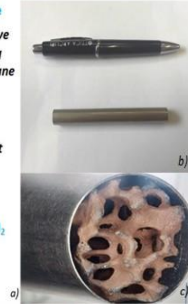
a) schematic view of the foam structured membrane reformer; b) Pd-Ag tubular membrane; c) Ni-Ru foam structured catalyst inserted in the lumen of the Pd-Ag membrane
