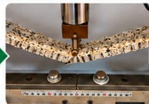
Three-point bending test Support distance: 304 mm
