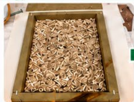
Larger sample production Mould filled with gasified wood pellets mixture
