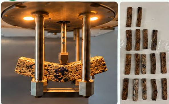
Three-point bending DMA at elevated temperature; cut specimens prepared from composite panels.
