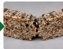
Failed specimen Typical fracture after maximum load
