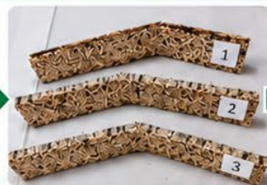
Test specimens (EN 310) Three 50 mm wide samples cut from the board
