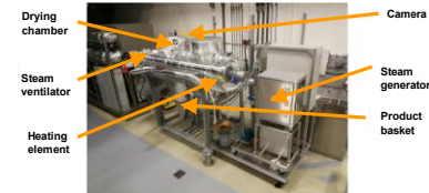
(b) Pilot-scale SHS drying unit to be upgraded as torrefaction unit at IGB (Germany)
