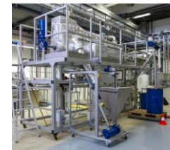
(b) Pilot-scale SHS drying unit to be upgraded as torrefaction unit at IGB (Germany)
