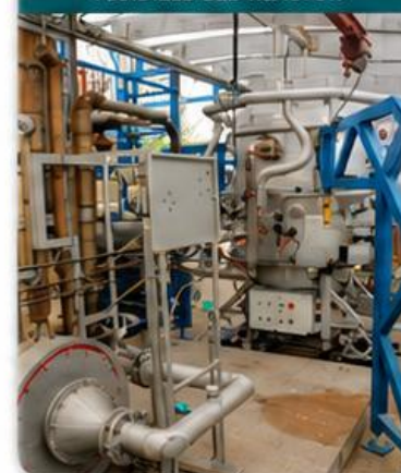
FLUIDIZED BED REACTOR
